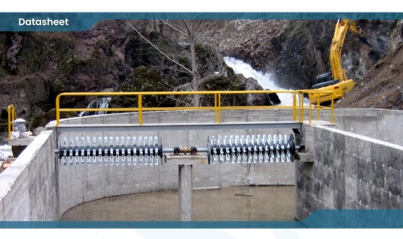
**Horizontal Shaft Surface Aerators with Brush**
